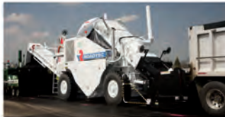
Material transfer vehicle Allows continuous paving
